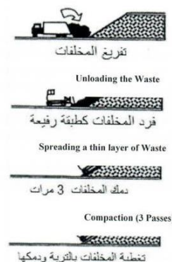
Figure (7): Covering Waste with Soil Cover followed by Compaction
